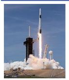
Falcon 9 is a partially reusable rocket. The first stage of the rocket is capable of re-entry and vertical landing. The first stage of the rocket has 9 Merlin engines. The second stage has 1 Merlin vacuum engine. Space X have had over 100 successful launches to date.
